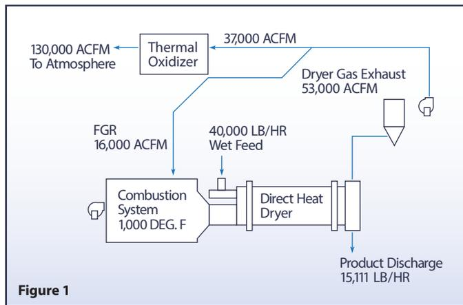
The direct heat dryer in the example is equipped with a combustion system having a dryer inlet gas temperature of 1,000 F. Based on this system, the dryer exhaust gas discharge volume would be 53,000 ACFM. The system is provided with a flue-gas recirculation system. This is included for two reasons:
